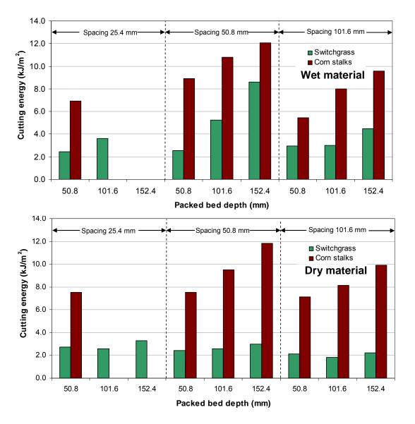
Figure 5. New surface area-based cutting energy of wet and dry switchgrass and corn stalks at different knife grid spacing and packed bed depths
