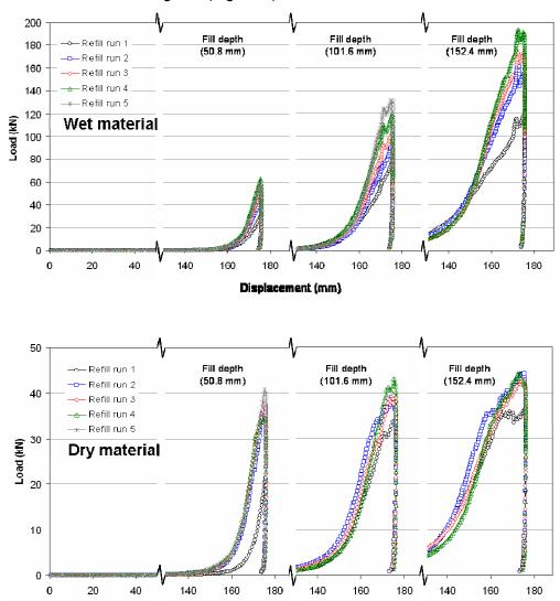
Figure 2. Typical load-displacement curves of wet and dry switchgrass at grid spacing of 50.8 mm
