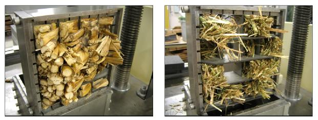
Figure 6. Cut product embedded in the knife grid annular space (50.8 mm (2") knife grid spacing).
