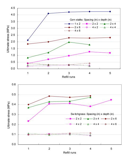
Figure 7. Ultimate cutting stress for corn stalks and switchgrass with different knife grid spacing and fill depths.
