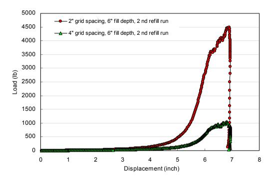
Figure 5. Typical load-displacement cutting characteristics of switchgrass under linear knife grid.
