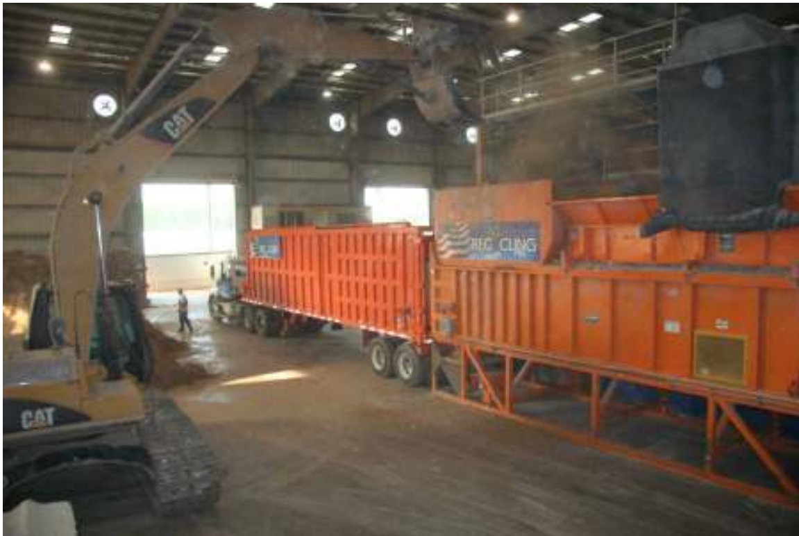
Figure 4. Compactor coupled with ejector-trailer
