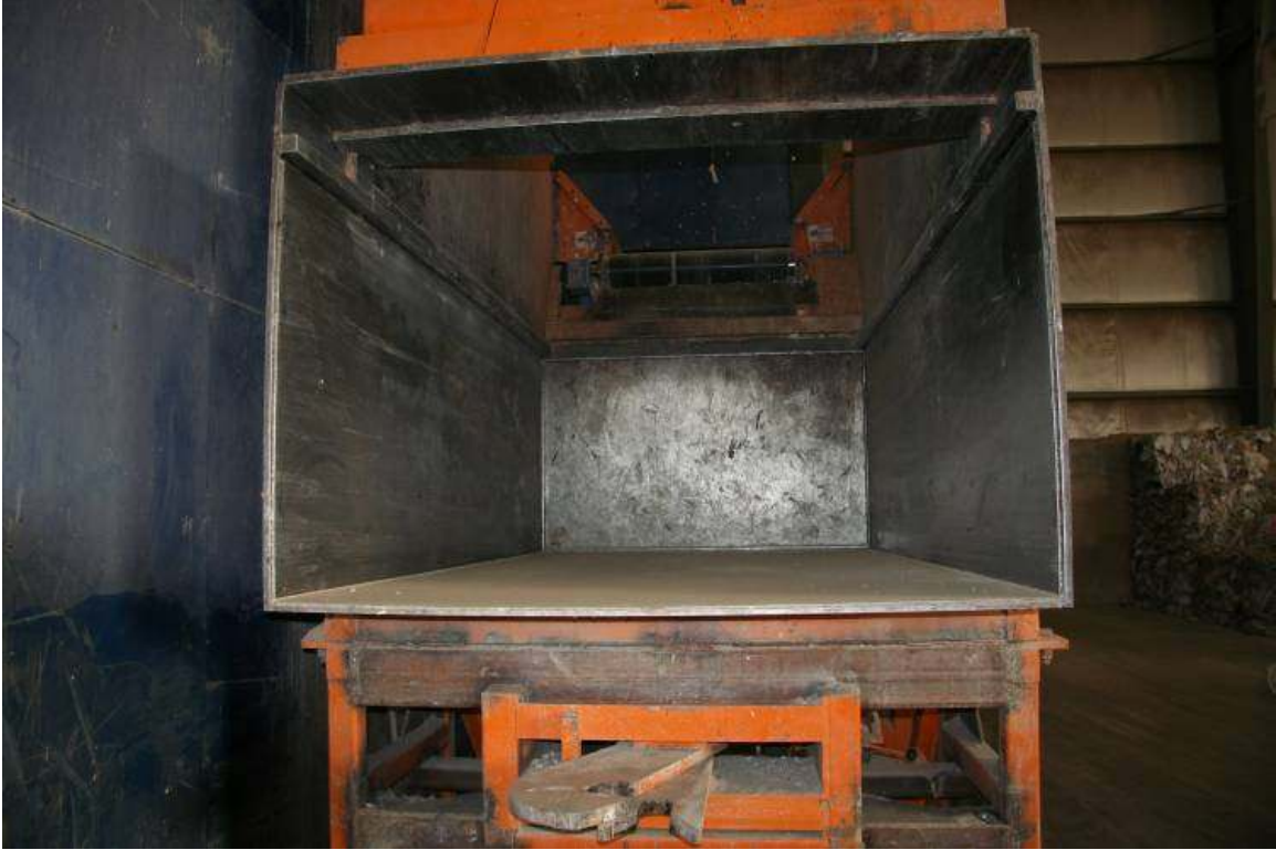
Figure 3. Marathon M-1475XW compactor charge chamber
