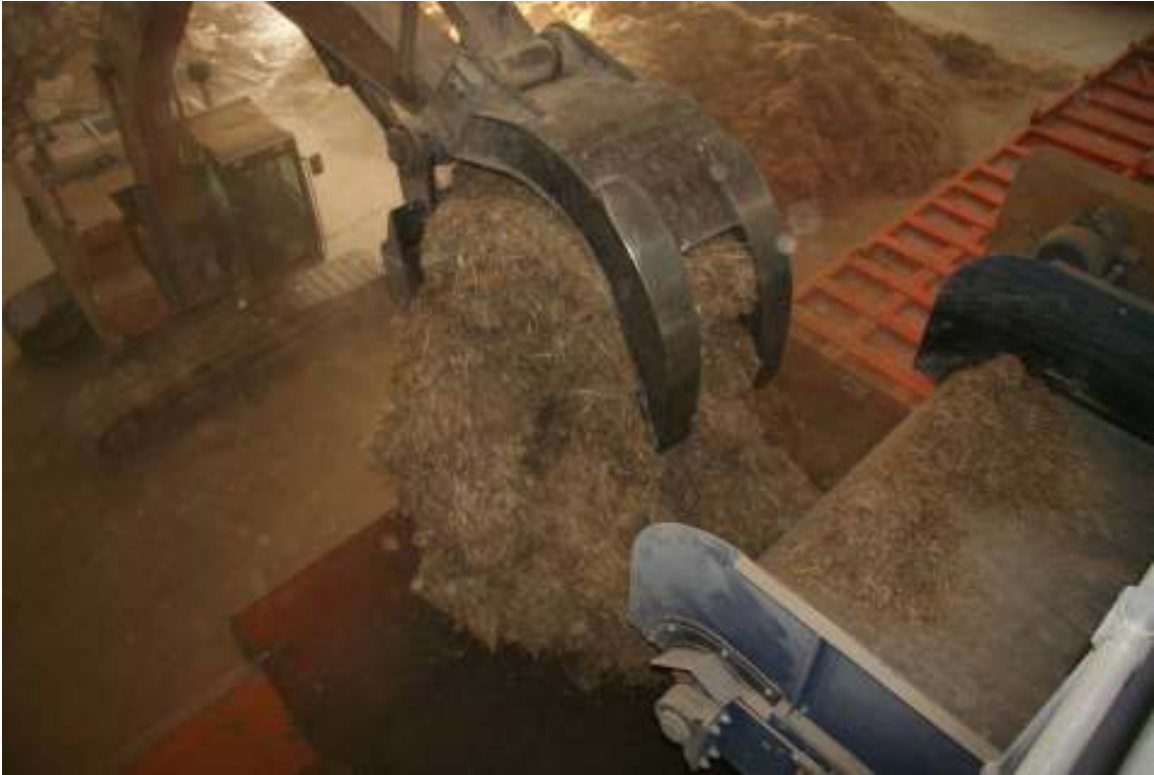
Figure 5. Compactor loading with excavator grapple
